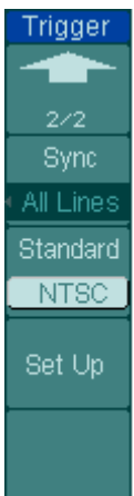
Figure 2- 59 Table 2- 35 The Alternate menu (Trigger Mode: Video, All Lines, Odd Field or Even Filed, Page 2/2)
